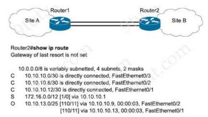
User traffic originating within site B is failing to reach an application hosted on IP address 192.168.0.10, which is located within site A. What is determined by the routing table?
