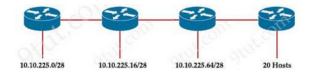
An engineer must add a subnet for a new office that will add 20 users to the network. Which IPv4 network and subnet mask combination does the engineer assign to minimize wasting addresses?
